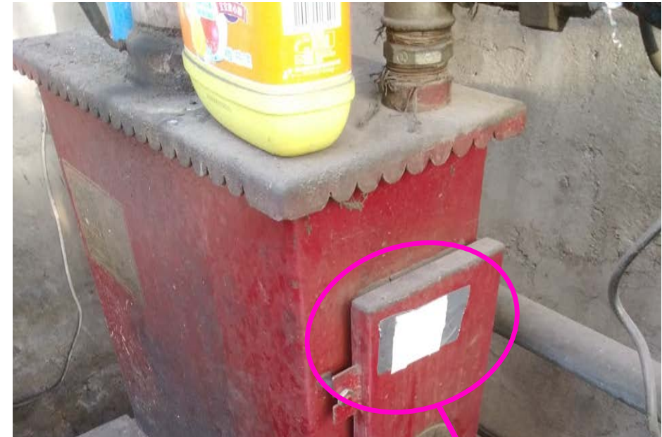
Stove Use Monitoring with Small Temperature Sensors
